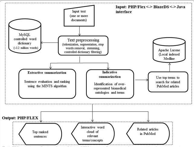
**Fig. 1** CERC system diagram. This shows the overall design of CERC. Input text is first preprocessed via segmentation, tokenization, stemming, and controlled dictionary filtering. Extractive summarization is performed using a new algorithm, the MINTS algorithm, a multi-stage algorithm for sentence extraction and ranking. A word-cloud based visualization method is used to represent term/concept distribution
