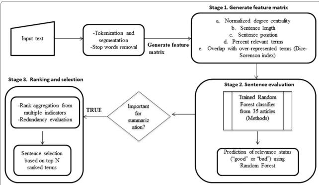
**Fig. 2** MINTS workflow for extracting salient sentences. MINTS uses a multi-stage framework that combines supervised learning techniques, individual characteristics of sentences (position, length, relevant terms) and network level characteristics (degree centrality) for extracting salient sentences
