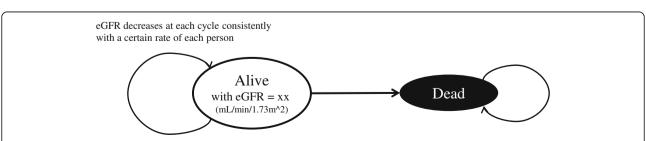
Fig. 2 State transition diagram of kidney function-based microsimulation (MSM-kf). The transition probabilities between states depend on eGFR value which constantly decreases at each time cycle with a certain rate
