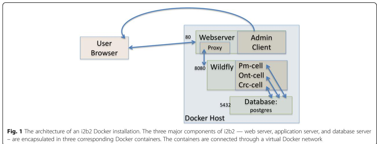
**Fig. 1** The architecture of an i2b2 Docker installation. The three major components of i2b2 — web server, application server, and database server — are encapsulated in three corresponding Docker containers. The containers are connected through a virtual Docker network
