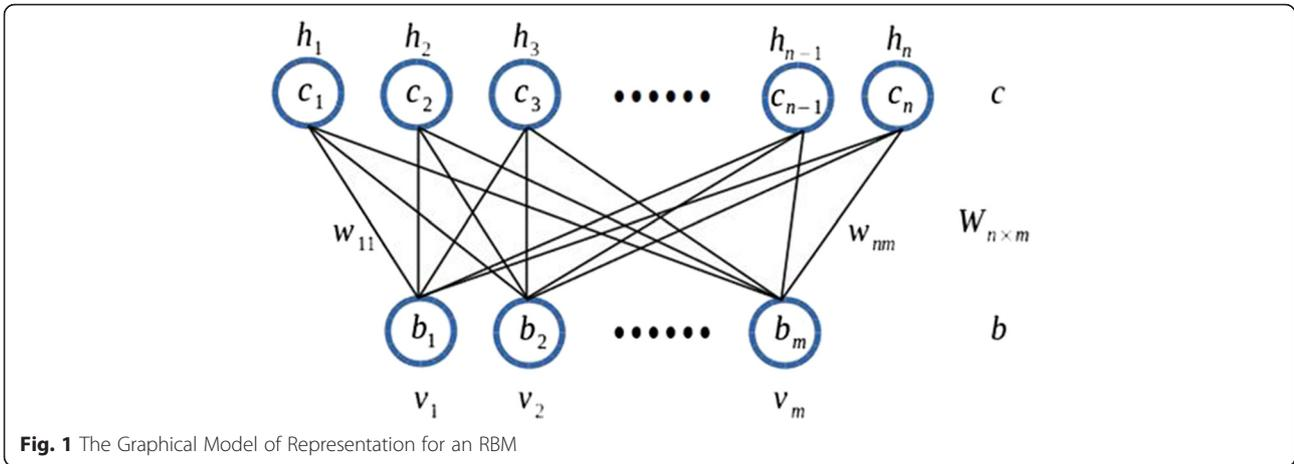
**Fig. 1** The Graphical Model of Representation for an RBM
