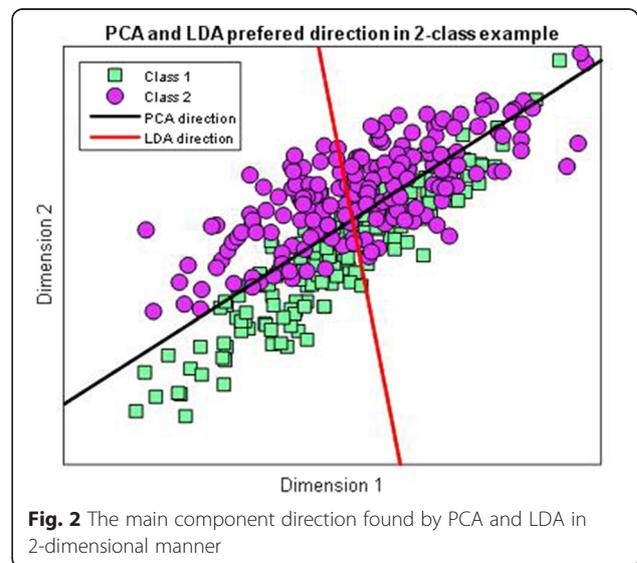
**Fig. 2** The main component direction found by PCA and LDA in 2-dimensional manner
