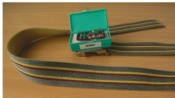
**Figure 1** Triaxial accelerometer sensor (*Freescale RD3152MMA7260Q*), sensor casing and belt. No skin contact is necessary for the sensor function
