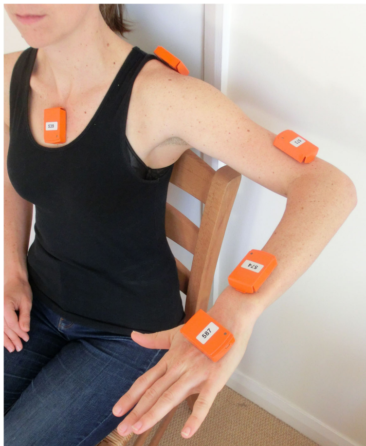
Fig. 2 Photograph showing the positions of the five IMUs attached with double-sided adhesive
