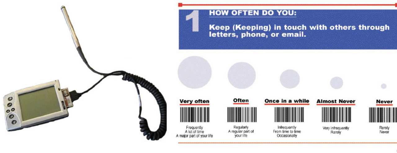
Figure 1 Overview of proposed system to collect outcome data electronically. A mobile computer (top left panel) accepting flash card adapters and running the Palm OS is connected to a barcode wand scanner to input outcome data. The survey questions and their answer fields are presented on paper (top right panel). Barcodes are associated with specific answer fields. The layout can be adjusted (type face, presentation of information etc.). Once collected electronically on the mobile computer, the information can be transferred to a PC database.
