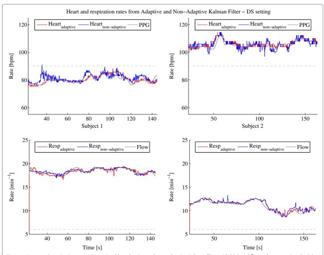
**Figure 4** Heart and respiration rates determined by adaptive and non-adaptive Kalman filter with PPG and flow reference using the DS setting. Heart (top) and respiration (bottom) rates determined by adaptive (red) and non-adaptive (blue) Kalman filter with PPG and flow reference (gray) using the DS setting for subject 1 (left column) and 2 (right column). The dotted gray lines indicate the starting frequencies of the heart and respiration rates defined in the setting at startup.
