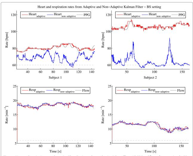
**Figure 5 Heart and respiration rates determined by adaptive and non-adaptive Kalman filter with PPG and flow reference using the BS setting.** Heart (top) and respiration (bottom) rates determined by adaptive (red) and non-adaptive (blue) Kalman filter with PPG and flow reference (gray) using the BS setting for subject 1 (left column) and 2 (right column). The dotted gray lines indicate the starting frequencies of the heart and respiration rates defined in the setting at startup.
