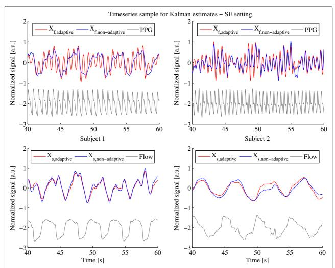
Figure 6 Internal states  $X_f$  and  $X_s$  determined by adaptive and non-adaptive Kalman filter with PPG and Flow Reference using the SE setting. Internal states  $X_f$  (top) and  $X_s$  (bottom) determined by adaptive (red) and non-adaptive (blue) Kalman filter with PPG and Flow Reference (gray) using the SE setting for subject 1 (left column) and 2 (right column).
