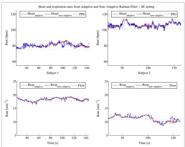
**Figure 3 Heart and respiration rates determined by adaptive and non-adaptive Kalman filter with PPG and flow reference using the SE setting.** Heart (top) and respiration (bottom) rates determined by adaptive (red) and non-adaptive (blue) Kalman filter with PPG and flow reference (gray) using the SE setting for subject 1 (left column) and 2 (right column). The dotted gray lines indicate the starting frequencies of the heart and respiration rates defined in the setting at startup.
