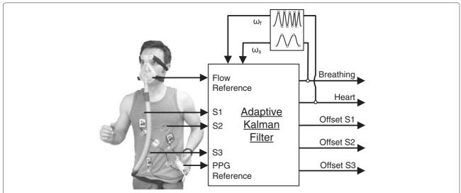
**Figure 1 Kalman filter sensor fusion.** Kalman filter sensor fusion (sensors: S1 to S3 with flow and PPG references) and vital signs extraction with frequency adaptation.
