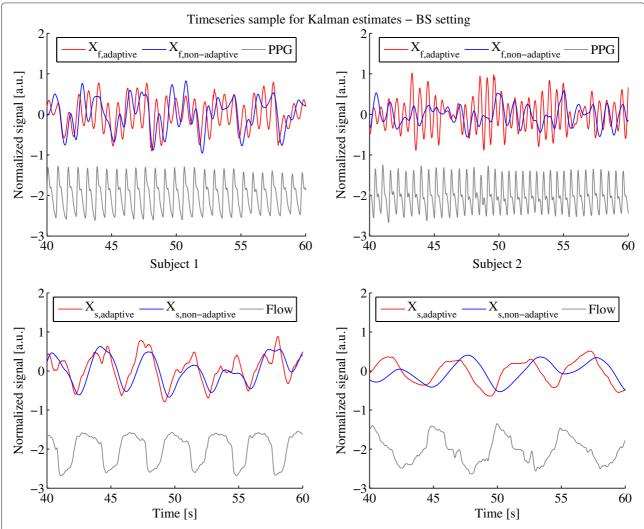
Figure 8 Internal states  $X_f$  and  $X_s$  determined by adaptive and non-adaptive Kalman filter with PPG and Flow Reference using the BS setting. Internal states  $X_f$  and  $X_s$  determined by adaptive (red) and non-adaptive (blue) Kalman filter with PPG and Flow Reference (gray) using the BS setting for subject 1 (left column) and 2 (right column).
