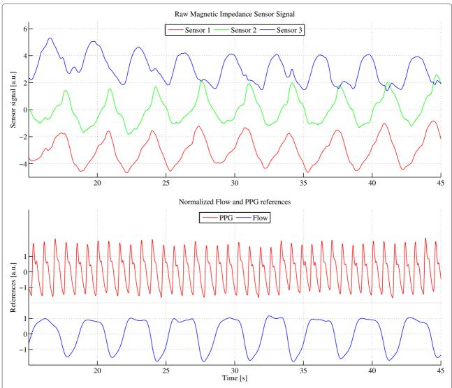
**Figure 2** Raw signal example with parallel Flow and PPG reference recordings. Raw signal of sensor 1-3 example (top with arbitrary units [a.u.]) with parallel flow and PPG reference recordings (bottom with arbitrary units [a.u.]) (30 s window).
