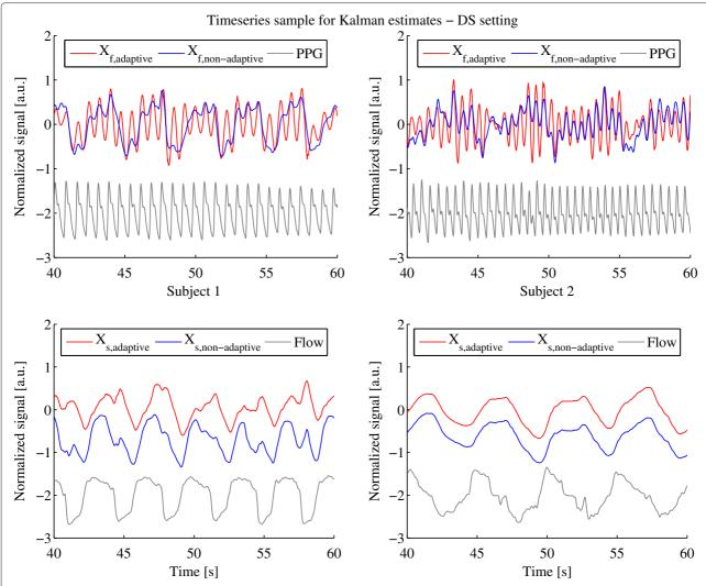
Figure 7 Internal states  $X_f$  and  $X_s$  determined by adaptive and non-adaptive Kalman filter with PPG and Flow Reference using the DS setting. Internal states  $X_f$  and  $X_s$  determined by adaptive (red) and non-adaptive (blue) Kalman filter with PPG and Flow Reference (gray) using the DS setting for subject 1 (left column) and 2 (right column).
